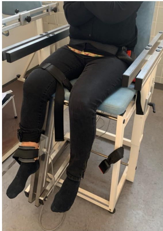
Figure 4. Setup for measuring leg muscle strength.
